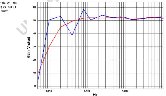
**Fig. 6** Shaketable calibration (blue curve) vs. MHD calibration (red curve)
