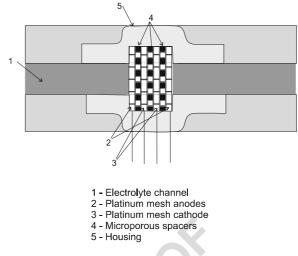
Fig. 1 Electrochemical transducer
