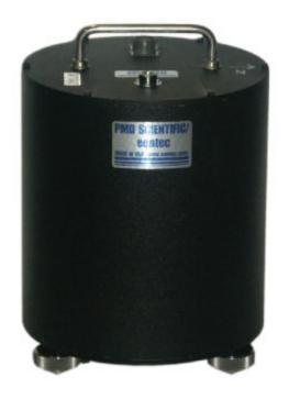
Each of the three identical sensors is equipped with a *force-balancing feedback* and the *noise floor is significantly reduced as compared to the previous models*. The sensors are offered in two application-dependent versions: EP-105SM with a higher clip level, and EP-105LN with reduced noise. Both versions have the same dynamic range, which is shifted up by approximately 10db in the 'SM' relatively to the 'LN' version. A single component instrument is also available.
