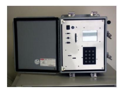
This extremely versatile seismic data acquisition system *can be configured from 4 to 32 channels*, all operating *synchronously up to 2,000 samples per second*. It is configured with an internal triaxial accelerometer (EA-120) in a weatherproof steel enclosure. Optional channels for external accelerometers are available.
