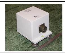
Like other *eentec* seismometers, the *SEISMINI* is extremely rugged which makes it ideal for field use. This seismometer *does not* require a mass lock, mass centering, or special installation equipment or procedures. The sensor has low power consumption, operates over a wide temperature range; it is waterproof up to 1m, and stays operational within a wide range of installation tilts.
